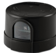
Twist lock long life photocontrol Multi-volt, fail-on, 8A at 120V and 5A at 277V HI-LL-127-15-BK-12
