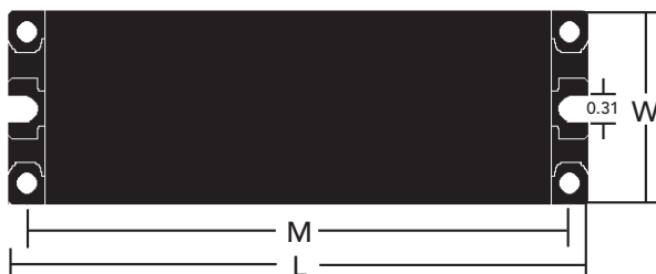
Bottom Ballast View
