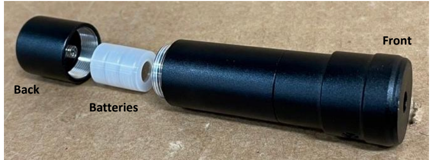
Step 1: Exploded view of laser pointer with batteries
