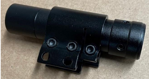
Step 3: Slide the laser pointer into the holder. Do not tighten any screws yet.
