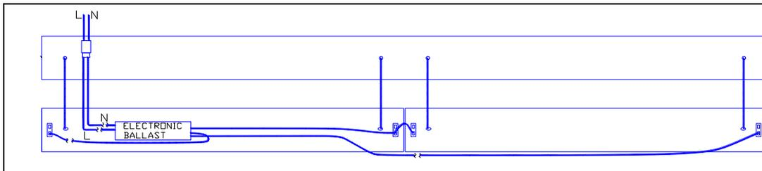
Existing fixture with fully wired retrofit kit.
