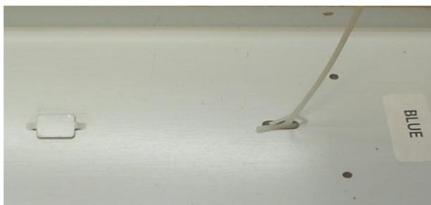
DIAGRAM 2 – Thread geartray tether into geartray.
