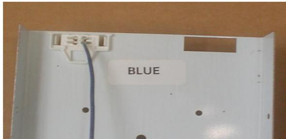
DIAGRAM 3 – Insert lampholder according to color labels.
