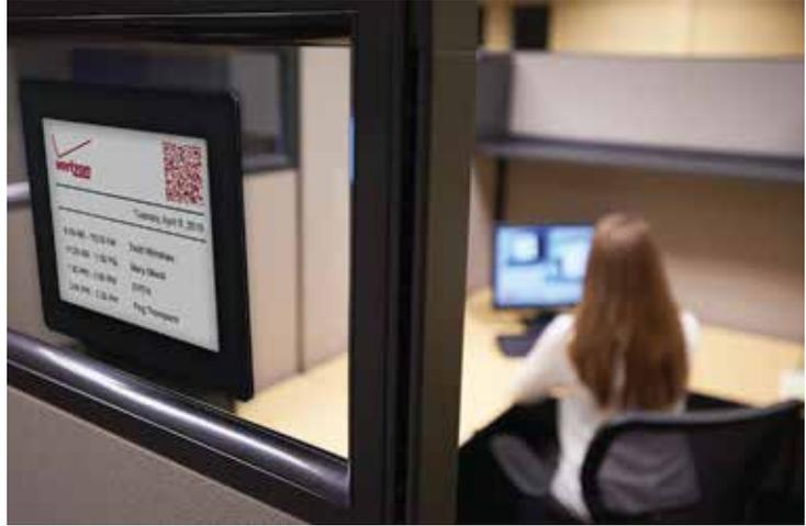
The room signs are updated wirelessly via RF communication designed to minimize battery usage. A sign's batteries are only activated when information changes, which allows batteries to last up to three years or 10,000 updates.
