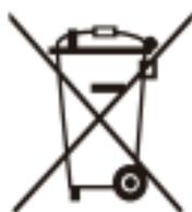
This marking on the product, accessories or literature indicates that the product and its electronic accessories (e.g. charger, headset, USB cable) should not be disposed of with other household waste.
