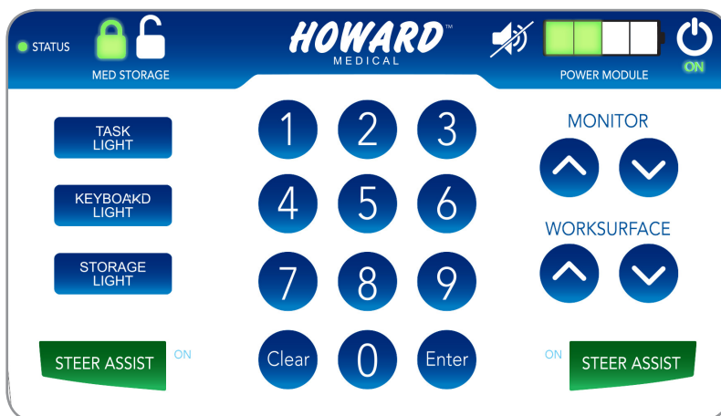
The HI-Care E's Easy Touch Membrane Keypad
