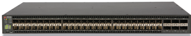
Figure 1: The Ruckus ICX 7750-48F features 48 1/10 GbE SFP+ ports and 6 40 GbE QSFP+ ports that can each be split into 4x10 GbE SFP+ ports. The front panel also displays the unit stacking ID.
