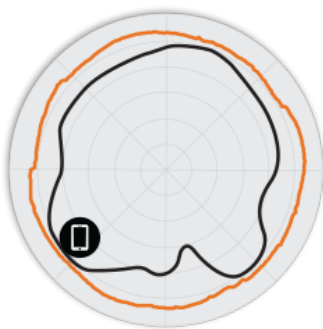
Figure 2. T310d 2.4GHz Azimuth Antenna Patterns
