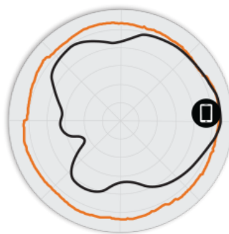
Figure 3. T310d 5GHz Azimuth Antenna Patterns
