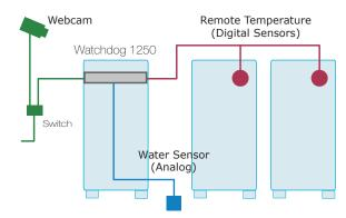
A Watchdog 1250 using remote temperature sensors to monitor multiple cabinets. A water sensor checks for water leaks, and a web cam provides remote images of the room.
