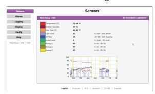
Current sensor readings and graphs are displayed or Sensors page of the web interface. Images from up four webcams are also displayed.
