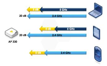
Enhanced receive sensitivity also has the added benefit of making 5Ghz coverage much broader and available to more clients who support the 5Ghz band, which helps to free up the over-used and crowded 2.4Ghz spectrum and allows higher speed radio communication on both spectrums. All in all, more intelligent access points combined with cloud-managed, cooperative control software enhance the Wi-Fi experience on any type of device, consumer-focused or not.
