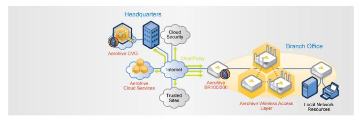
Besides extending the corporate network to remotely connected users and devices, Aerohive branch routers support full enterprise-class enforcement for BYOD, including client classification and full stateful firewall.
