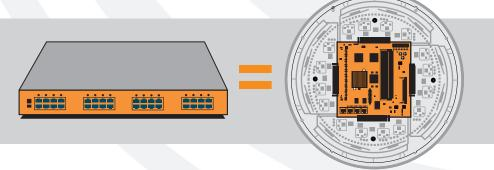
The Xirrus Wi-Fi Array distributes the processing power and network intelligence to the network edge to increase performance and quality of experience. Antiquated thin AP + controller architectures backhaul everything to a central controller located back in the network, creating delay and jitter.
