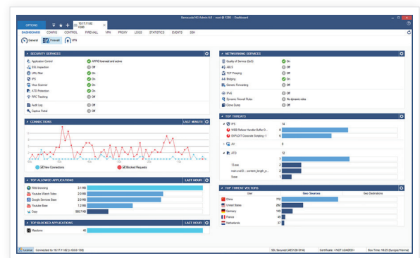
The Barracuda NextGen Firewall F-Series' dashboard provides real-time information and summaries of what is going on in an organization's network.
